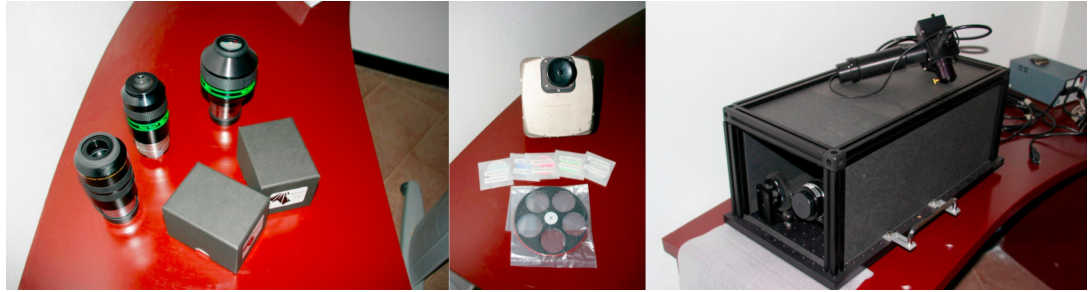
Figure 6. The Antola Observatory instrumentation. On the left the set of eyepieces, in the center the SBIG camera and the filters, on the right the FLECHAS fiber-fed spectrograph.
