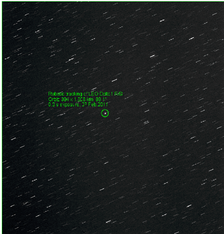
Figure 1. TFRM robotic observation of the LEO Delta1 R/B, encircled in green. Orbit 304, distance 1608 km, inclination 89.1 degrees. The image was taken on Feb 7th 2011, with an exposure time of 0.3 second.
