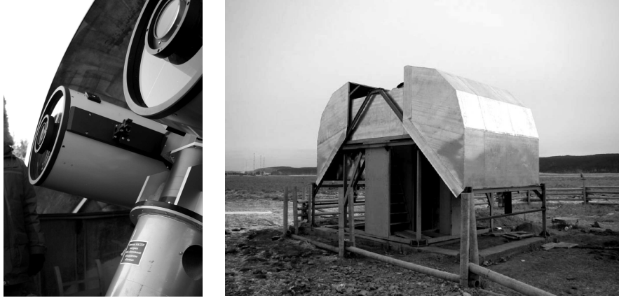
Figure 2. Left: MASTER II telescope assembly at Kourovskaya astronomical observatory, with no photometric units and CCD attached. Right: custom steel enclosure for Irkutsk university polygon in Tunka valley.
